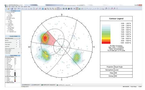
Kinematic analysis, planar sliding using pole vectors, daylight envelope, 30 degree friction angle, 70 degree slope angle.
