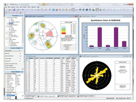
Dips file showing input data spreadsheet, contour plot with overlaid symbolic pole plot, rosette plot and chart.
